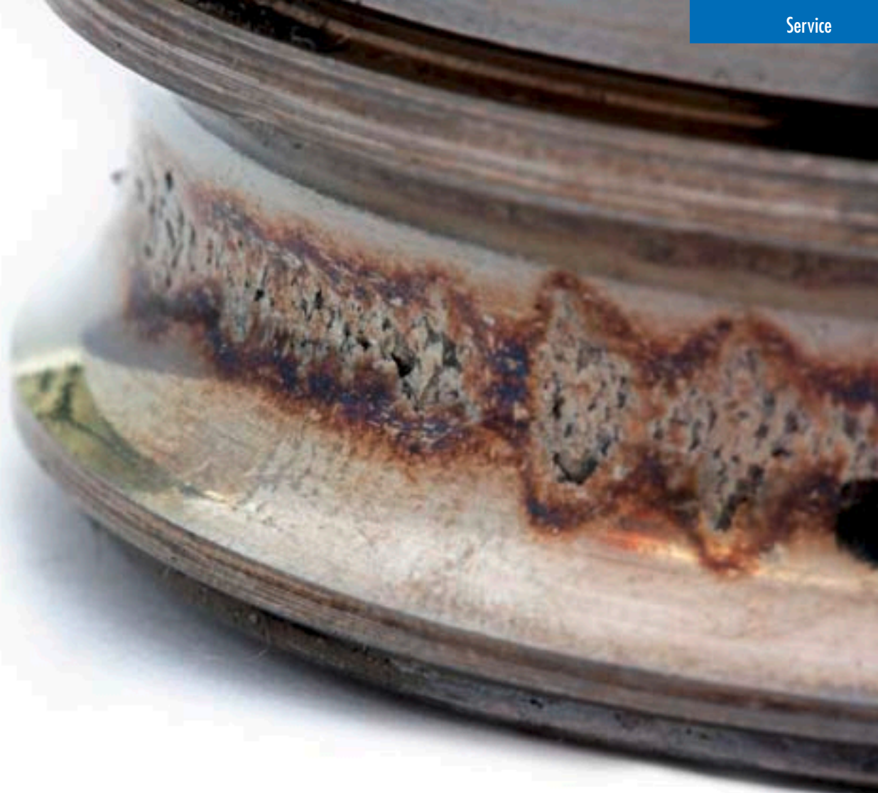
Figure 3: A lack of lubrication of the ball bearings led to the damage occurrence.
